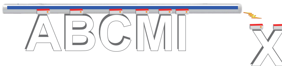
3. Hook up the track to the suspension cable and put the power cable in place.
