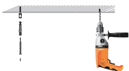
1. Drill screw holes from the ceiling
